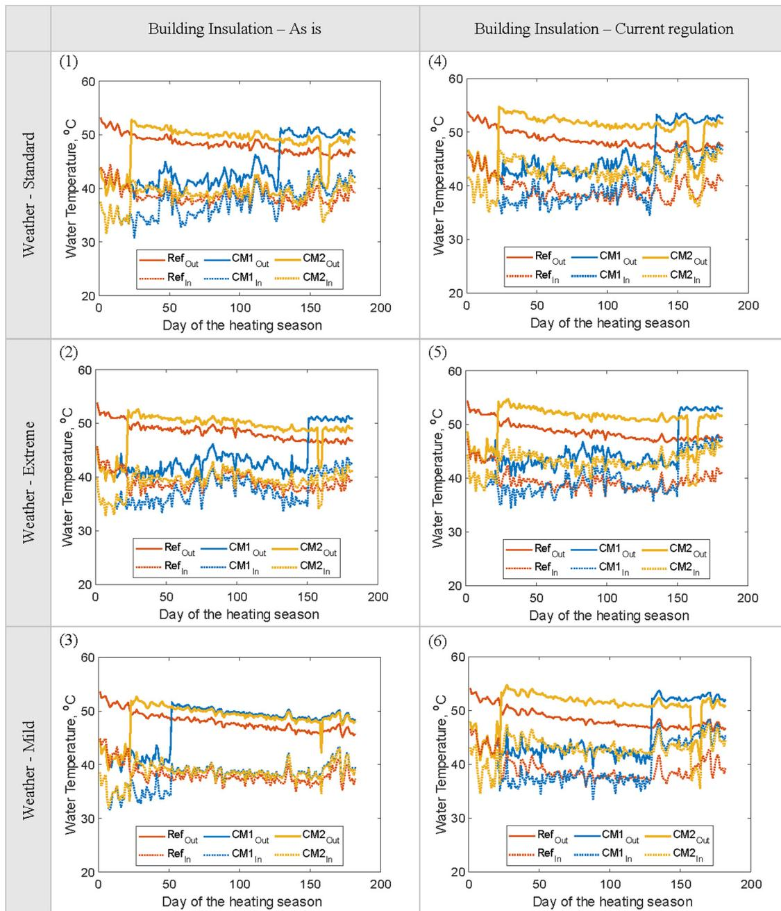
**Fig. 15.** Comparison on the daily average inlet and outlet temperature for the BTES subsystem in the heating season among different BTES operation strategies at different weather and building insulation scenarios; Ref- overall control, CM1- zonal control, CM2- time-scheduled combined control.
