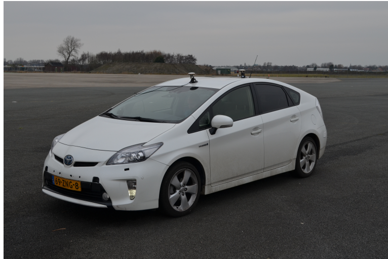
Figure 1. The Toyota Prius used for this work (the two devices on the roof of the vehicle are part of the Spatial Dual GPS).
