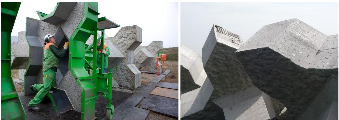
Figure 6-7. Eco Xbloc® mould and different concrete surfaces specifically prepared to enhance flora and fauna habitats
