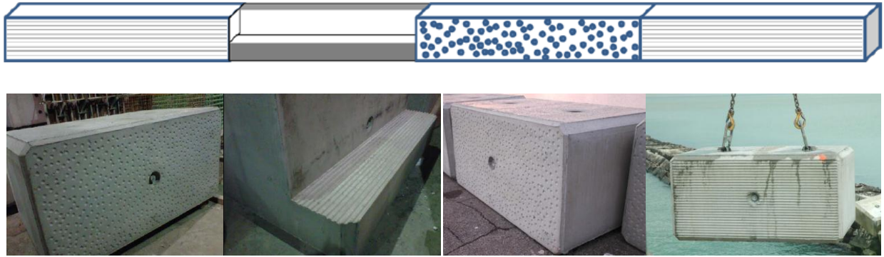
Figure 6-15. USACE designed green concrete toe units for Cleveland Harbour breakwater, Ohio, USA.
