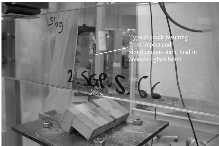
Fig. E.25 Typical fracture pattern in 3.SG.A beam after impact in two outer layers while simultaneously applying a static load. Disregard the ‘S’ in the name – this specimen turned out not to be heat strengthened.
