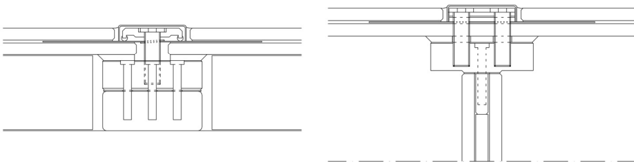
Fig. A.37a, b ATP façade panel – roof plate joint; vertical sections in two perpendicular directions.
