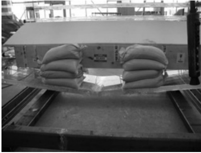
Fig. 5.10 Post-failure behaviour of an SG laminated glass plate.
