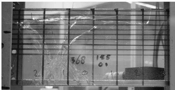
Fig. 9.10a Typical fracture pattern in slim beam after initial failure. A portion of the beam (at the top) remains unbroken.
