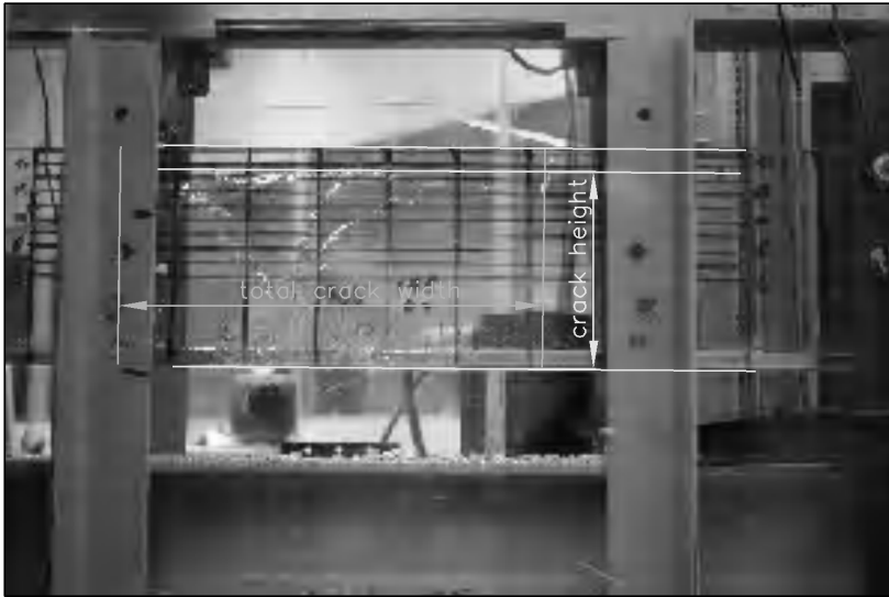
Fig. H.5 Photograph of initial crack pattern of specimen I-01 in Autocad. Determination of crack related results crack height and total crack width.
