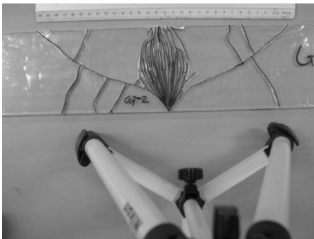
Fig. G.2a Specimen G7-2 with highlighted cracks.
