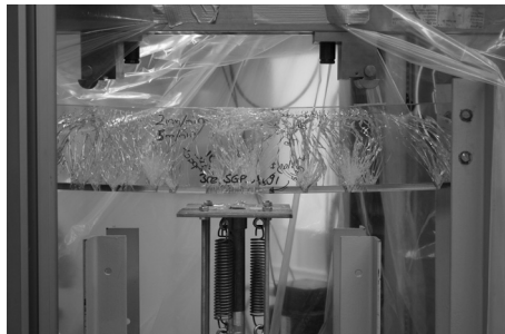
Fig 7.15c Typical final failure in 3re.SG.A specimen (after resistance test on specimen with model level III damage).
