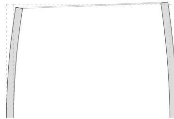
Fig. A.2 Possible shape distortions in the ends of glass tubes (exaggerated).
