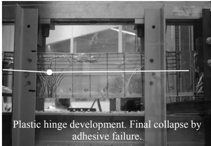
Figure 9.13a Plastic hinge determines 2 nd LTM in GB368 bonded reinforced glass beams. Maximum theoretical capacity is 3.59 kNm.
