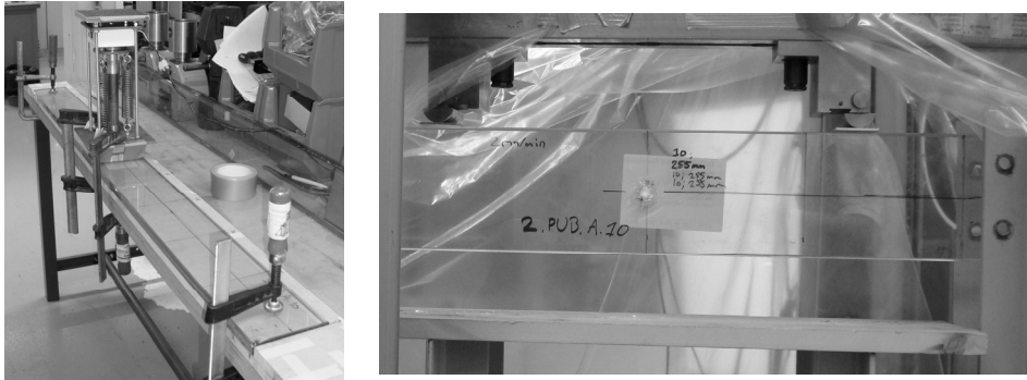
Fig. E.5a, b 2.PVB.A specimen before being subjected to side impact, and after side impact in 4-point bending test set-up.
