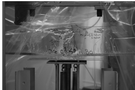
Fig. E.13 Typical post-failure behaviour of a GB368 bonded, reinforced specimen (pd 3re.GB368.A_2).
