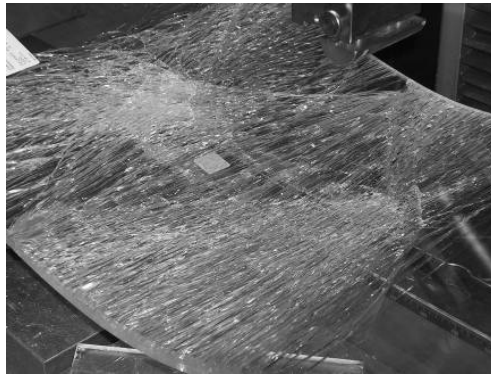
Fig. A.10 Scale model of ATP façade panel design crack pattern after four-point bending test.
