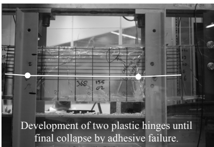
Figure H.6a – d (top to bottom) Crack development in specimen I-02.
