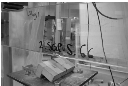
Fig 7.8b Typical model level I damage in 2.SG.A specimen.
