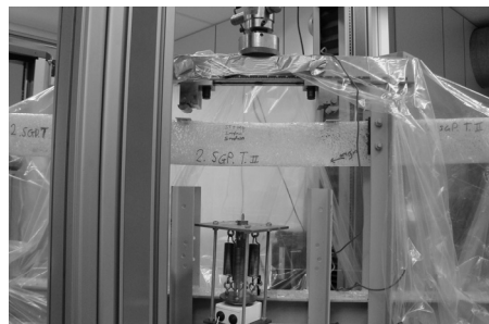
Fig 7.10b Typical final failure in 2.SG.T specimen (after resistance test on specimen with model level II (=III) damage).
