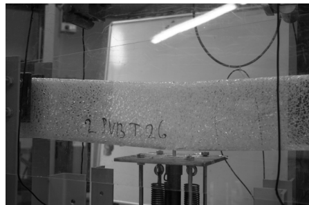
Fig 7.4c Typical final failure in 2.PVB.T specimen (after resistance test on specimen with model level II (=III) damage).
