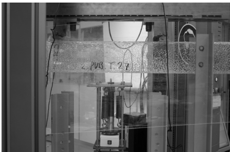
Fig 7.4b Typical model level I damage in 2.PVB.T specimen.
