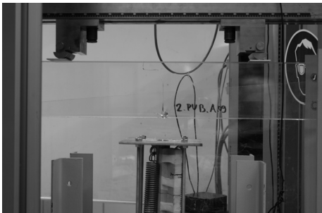
Fig 7.2b Typical model level I damage in 2.PVB.A specimen.
