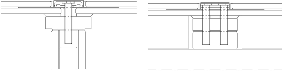
Fig. A.34a, b ATP purlin – roof plate joint; vertical sections in two perpendicular directions.
