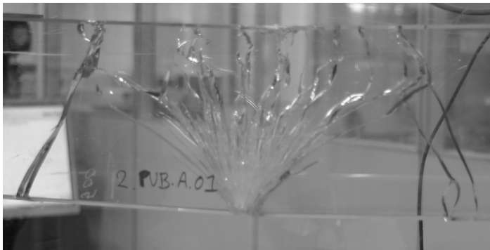
Fig. 9.6c Fracture pattern at initial failure in a double layer annealed glass beam tested in 4-point bending, with no predamage (level 0).
