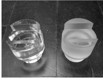
Fig. A.11 Flame polished (left) and machined (right) PMMA joint components.
