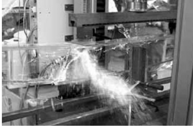
Fig. 8.14b Explosive final failure of the compression zone in a reinforced, post-tensioned T-shaped glass beam.
