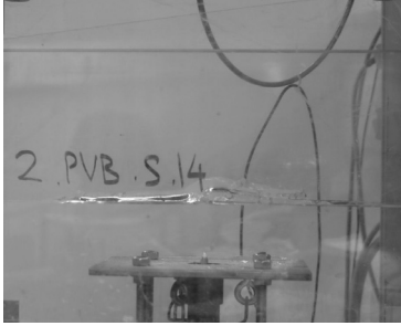
Fig. E.12 Typical physical damage in heat strengthened as caused by an 3.77 J impact from the impact device (specimen pd 2.PVB.S_1).
