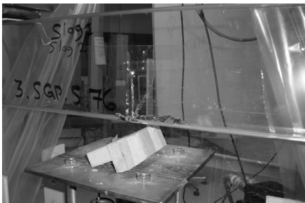
Fig 7.11b Typical model level II damage in 3.SG.A specimen.
