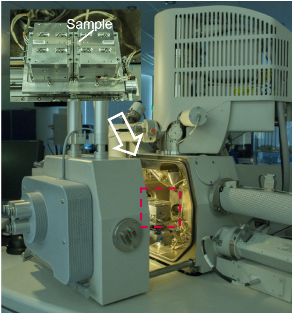
Figure 6. The tensile stage placed inside the FEI Quanta 600 ESEM. The high-vacuum compatible tensile stage can be tilted ( +5^\circ to -75^\circ ) with the SEM sample stage.
