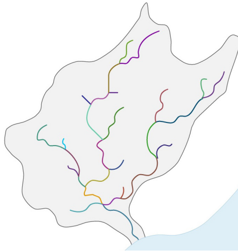
Figure 6.3: Artificially created example of river reaches in the HydroSHEDS/GloRiC dataset. A river reach, indicated by its own colour, is defined as a stretch between two tributaries, or between the start/end of the network and a tributary. The grey contour indicates the watershed. The river ends at the sink, a lake or ocean, indicated with the blue area. We can see that no bifurcations exist in this dataset.
