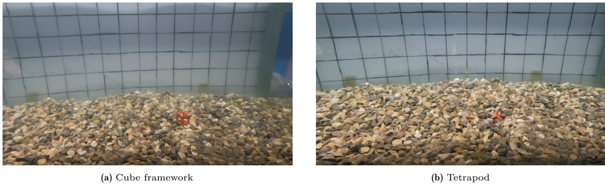
Figure 5.4: Concepts on the stone layer in wave flume during the stability test
