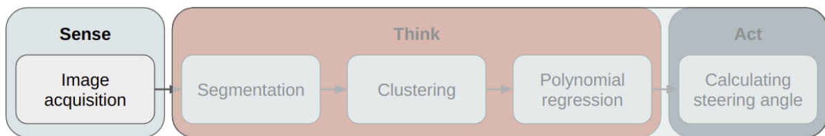
Figure 3.1: The flow scheme of the Sense-Think-Act robot model
