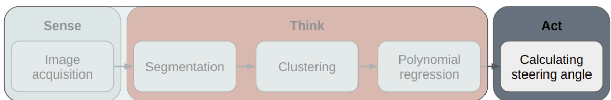
Figure 5.1: The flow scheme of the Sense-Think-Act robot model
