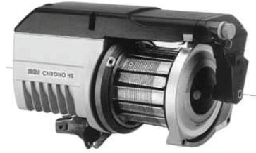
Figure 93. Fournisseur with yarn. Tether enters on left.
