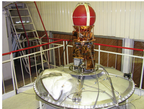
Figure 209. YES2 integrated with Foton battery pack (Samara)
