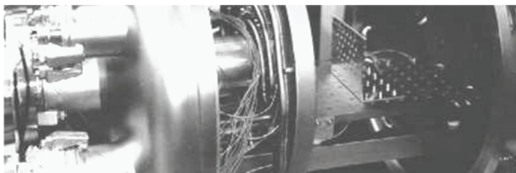
Figure 83. Sample holder in Bake-Out facility
