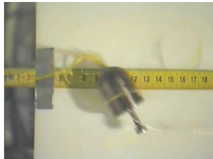
Figure 69. After ripstitches break, the mass floats rather than jumping back
