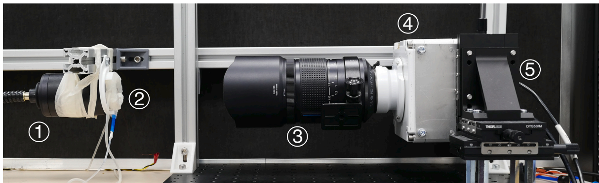
Fig. B.3. Experimental setup for vibration characterization: (1) light source, (2) multimodal ring under test, (3) lens, (4) camera, and (5) positioning system composed of three translation stages (DTS50/M, Thorlabs).
