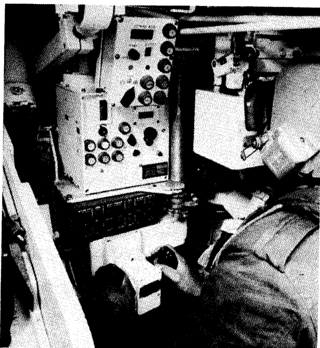
Elbit's Tank Fire Control System (TFCS) installed in the Merkava tank
