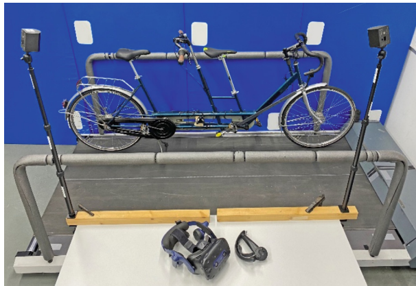
Fig. 3. 'Physical Prototyping Environment' – tandem on a treadmill, VR headset and controller.
