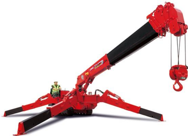
Spider crane. Limit 3T x 3.4m. See figure 102. (Unicranes, 2020)
