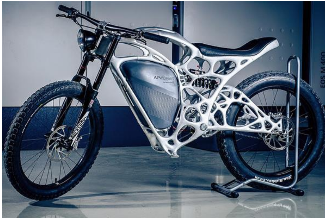
Light Rider: The 3D printed TO motorcycle (Grolms, 2016)
