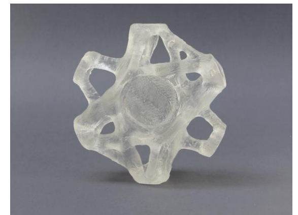
Casted TO node for heavy structure (Damen, 2019)
