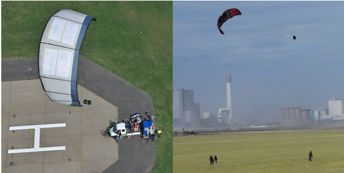
Figure 2.11: The 20kW ground station fitted with the regular 25m 2 kite at the Valkenburg test site (left, photo: Max Dereta) and with a small 14m 2 kite for peak wind speeds up to 17m/s at the Maasvlakte 2 test site (right) (van der Vlugt et al., 2013).
