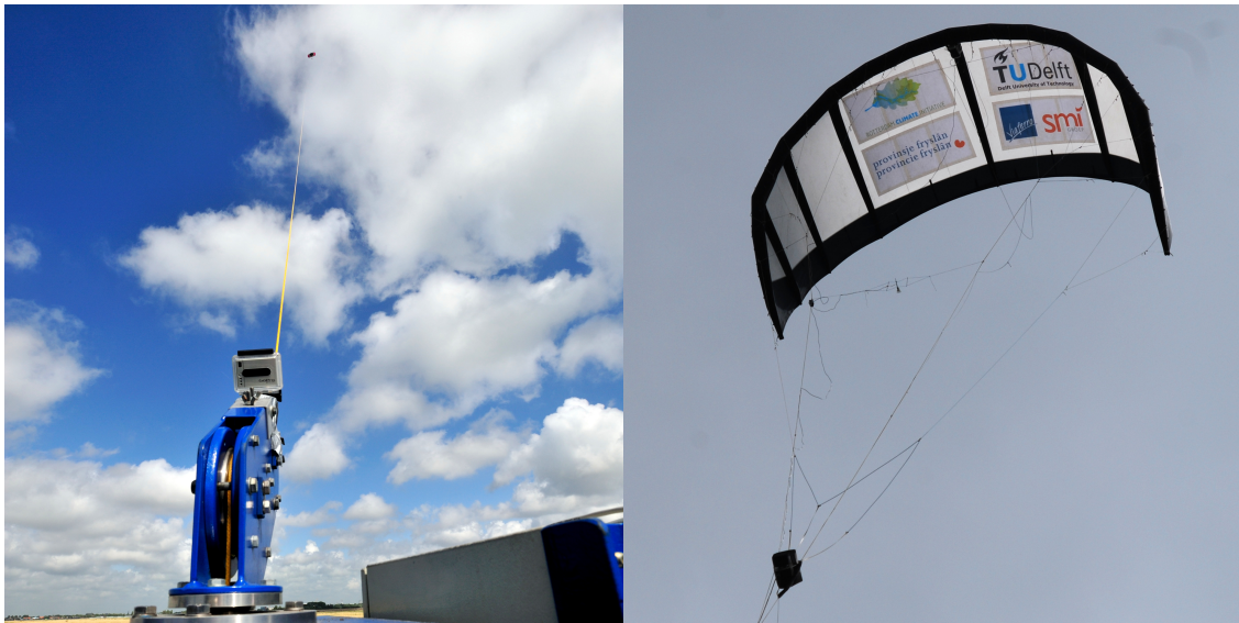
Figure 2.12: Swivel together with the tether in the sky(left) and the Mutiny, bridle system and kite control unit(right) (van der Vlugt et al., 2013).
