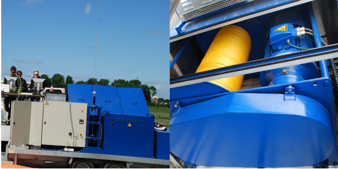
Figure 2.13: Ground station on trailer with tether running into the sky(left) and drum/generator module mounted on transverse sled(right) (van der Vlugt et al., 2013).
