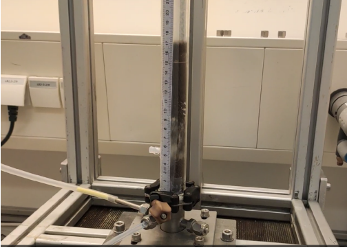
(a) The experimental setup used to determine the fluidization parameters of the seeds.
