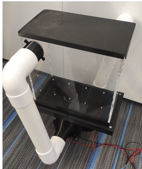
(b) Spouted bed configuration with recirculation pipes attached.
