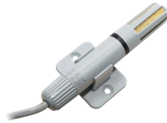
Figure 13: AM2315C combined temperature and humidity sensor. source: [35]
