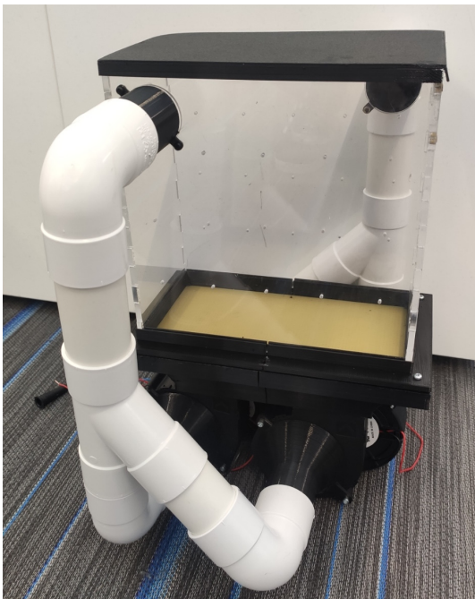
(a) Bubbling bed configuration with recirculation pipes attached.
