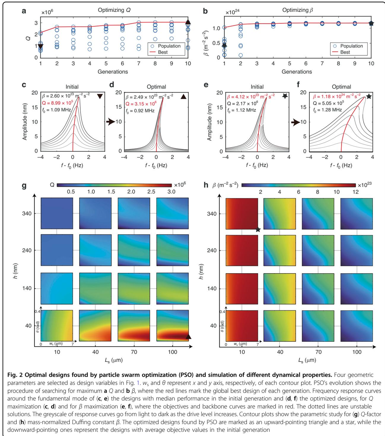
in Fig. 2a, c, d) or maximizing the mass-normalized Duffing constant  $\beta$  (shown in Fig. 2b, e, f) of the fundamental mode. We emphasize that a maximum  $Q$  or  $\beta$  does not necessarily result in the best performance for all applications of nanomechanical resonators. We choose these optimization objectives as examples to
