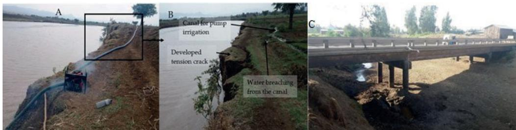
Figure 2.14. (A) Water extraction with a diesel pump for irrigation, (B) Irrigation canal to transport extracted water, which has been breached, and adjacent failing banks and (C) Ribb River during the dry season. The farmers excavate holes in the sandy river bed to get water for cattle and backyard irrigation. The photos were taken during a field campaign in April 2017.
