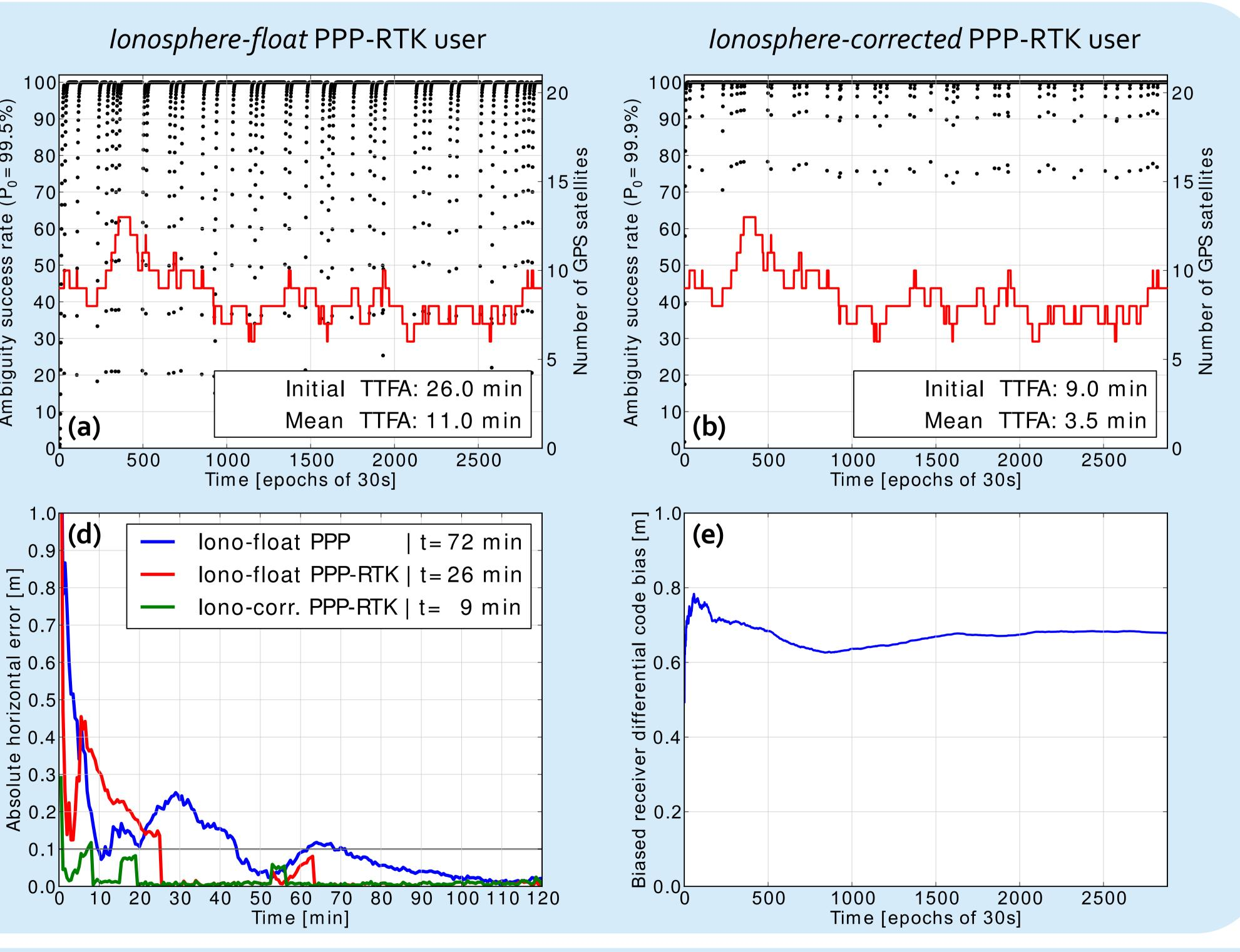
The **ionosphere-float model is weak in terms of IAR** due to the increased number of unknown parameters. • **Precise ionospheric corrections** can significantly reduce the convergence time.
