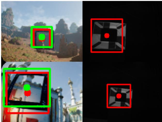
Fig. 3: On the left, the test set of the simulation dataset, in green is the label and in red are results of Gatenet. On the right, two images captured by the AI-Deck camera. Again in red the output of the network, no labels are present for these images.
