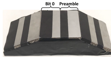
Fig. 22. The object-ID (preamble + ID value “0”) that is attached to all three parts of the object.
