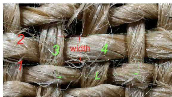
Figure 4. The geometries used to measure yarn width (lines 1, 2) and twist (lines 3, 4 and segment L).
