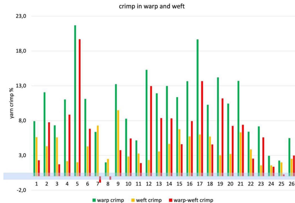
Figure 11. Crimp values in the warp are higher than in the weft in 96% of the cases.
