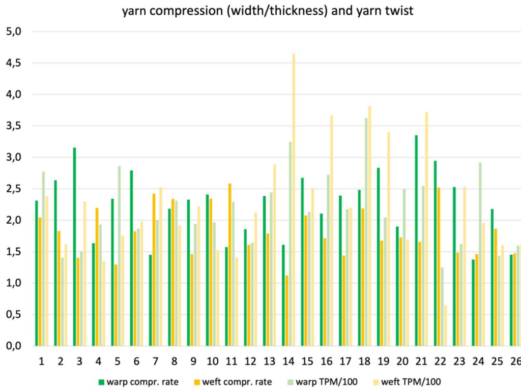
Figure 10. The yarn compression on the z axis of the textile (yarn width over thickness) and TPM. Higher TPM implies lower yarn compression.
