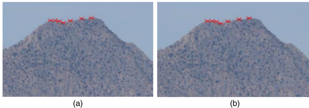
Fig. 3 Selected tracking points for the JER mountain peak target: (a) initial frame and (b) the following frame.
