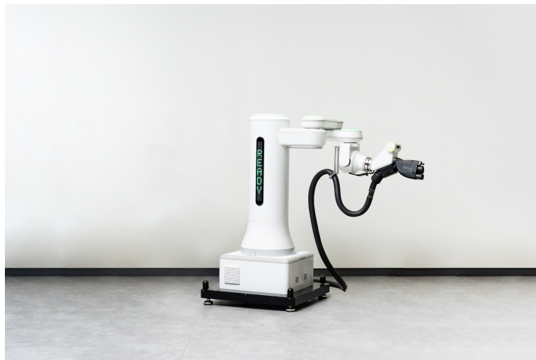
Figure 2.11: ACR developed by Hyundai Robotics Lab. [98]
