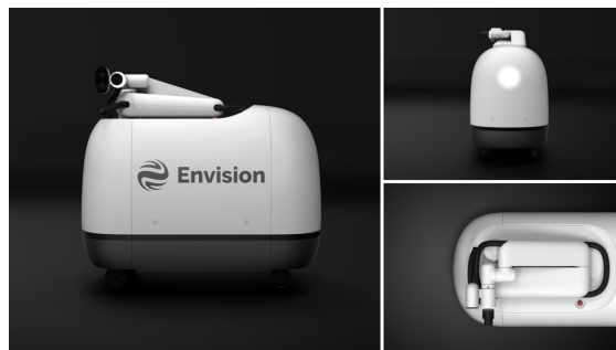
Figure 2.19: Mochi Charging Robot Developed by Envision Group [53]
