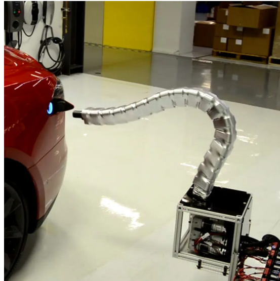
Figure 2.8: Bionic Charging Robot Prototype Developed by Tesla Motor Company [182]
