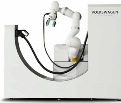
Figure 2.10: E-smart Connect Charging Robot Developed by Volkswagen AG and Kuka AG. [90]
