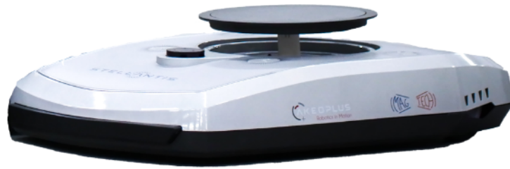
Figure 2.5: Inductive Charging Robot Developed by EFI Automotive [48]
