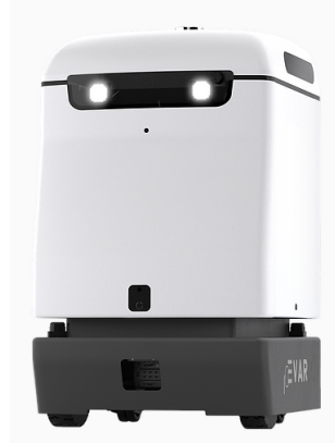
Figure 2.18: Parky Charging Robot developed by EVAR [71]
