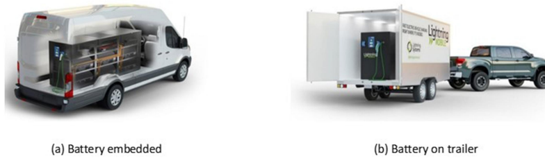
Figure 2.12: Categories of Battery Integrated Vehicles [25]
