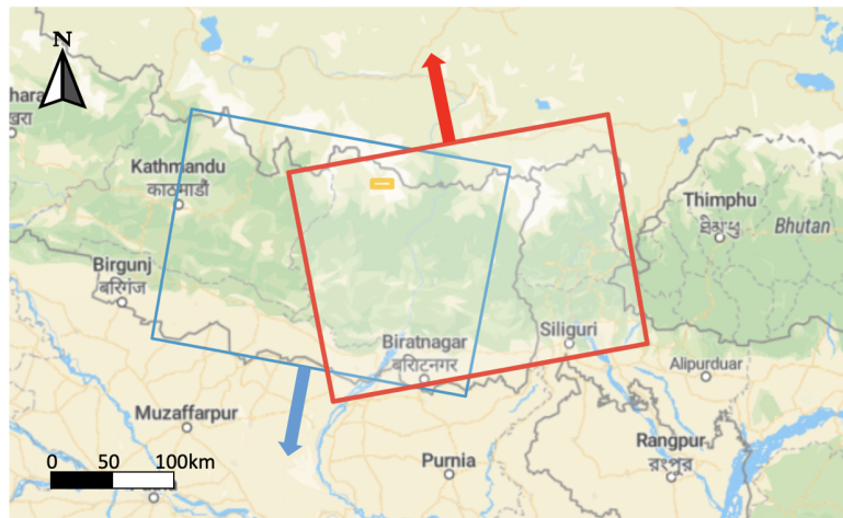
Figure 28: Footprint of the ascending (red) and descending (blue) path for the AOI Imja Lake (yellow)
