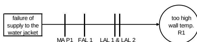
Figure 4: Scenario 'too high wall temperature R1' by failure of the water jacket cooling
