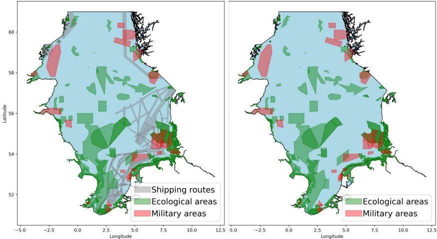
Figure 32. Forbidden areas for energy island construction (left) and for electricity cables and hydrogen pipelines placement (right). Ecological areas are in green, military zones in red and shipping routes in grey.
