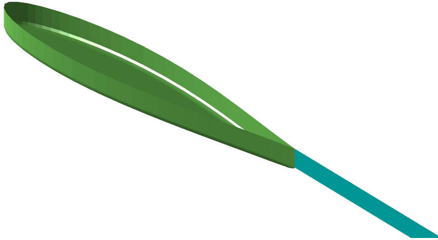
Figure 8.1: Beukelman wing ( \beta = 4 ) with a wake surface attached to the trailing edge of the wing only
