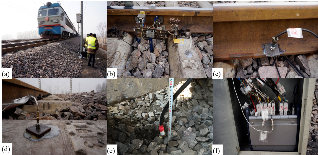
Fig. 15 Field testing: (a) field test location; (b) displacement sensors; (c) accelerometer on rail; (d) accelerometer on sleeper; (e) accelerometer embedded in ballast layer; (f) data acquisition system
