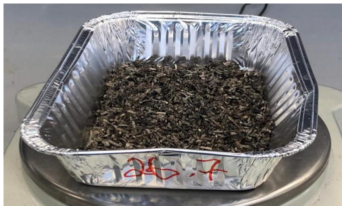
Image 8: shows the recovered subsamples from sample 3 (3.1 as 26.1, 3.2 as 26.2, 3.3 as 26.3) show a consistency of glass mixed with dark grained particles. The rest of the subsamples (3.4 as 26.4, 3.5 as 26.5, 3.6 as 26.6, 3.7 as 26.7) show a mix of metal filaments of a grey brownish color (likely copper mixed with tin).
