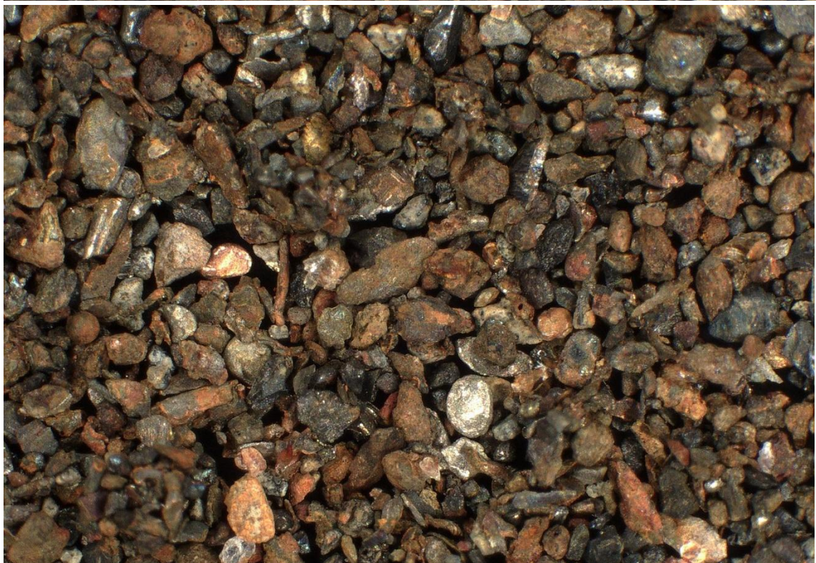
Image 9: shows the pictures made by the optical microscope Keyence VHX-7000. (The upper picture the results after leaching with citric acid and the lower picture after HCL.). In the upper picture the particles appear to be a mix of oxidized materials, with a relatively rough texture and a predominately reddish-brown residue, likely indicating the presence of rust. Some particles exhibit a shiny, reflective surface, possibly metallic inclusions. The bottom image has a similar composition to the upper one, but the particles appear cleaner (less rust). More visible metallic inclusions can be seen scattered throughout the bottom sample.
