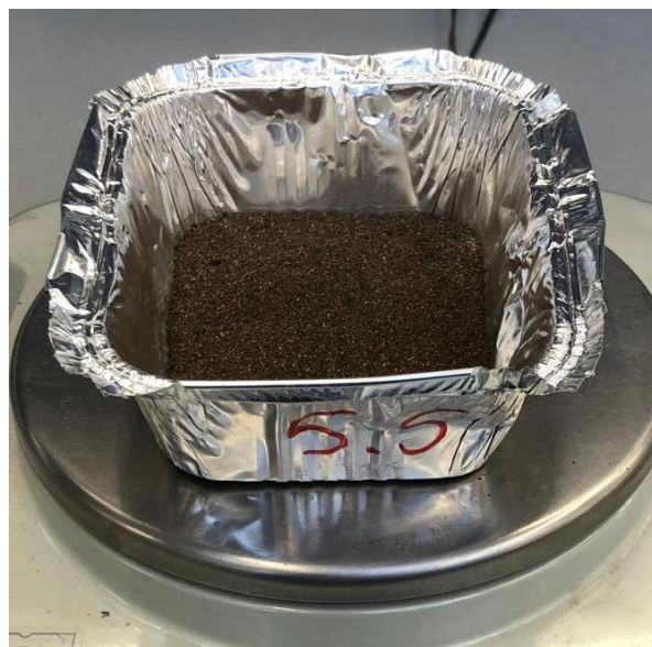
Image 6: shows the recovered subsamples from sample 1 (1.1 (as 5.1), 1.2 (as 5.2), 1.3 (as 5.3) consisting mostly of sand particles (yellow color), in sample 1.3 (as 5.3) you can see some dark-colored particles mixed in the sand. In subsample 1.4 (as 5.4) shows mostly copper particles mixed with small amounts of sand and in 1.5 (5.5) the subsample shows a mostly black-reddish color from the copper particles.
