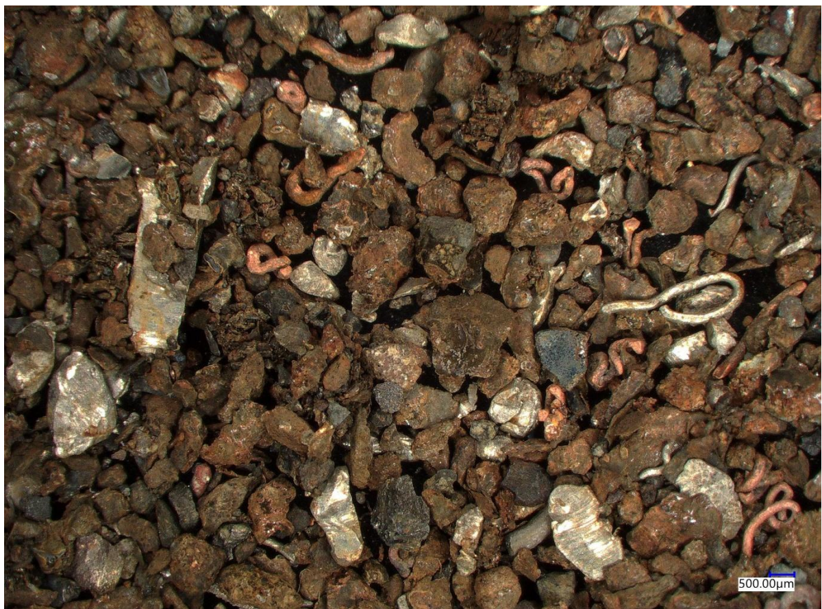
Image 10: shows the pictures made by the optical microscope Keyence VHX-7000. (the upper picture the results after leaching with citric acid and the lower picture after HCL.) The surface texture of the particles in the upper image appears rough and coated with a significant amount of oxidized layer (rust). There are also noticeable elongated, wire-like fragments among the particles, likely remnants of metal wiring. The bottom image appears to have a greater number of shiny metallic fragments exposed with a higher contrast between the oxidized and metallic components, with more distinct metal pieces visible.
