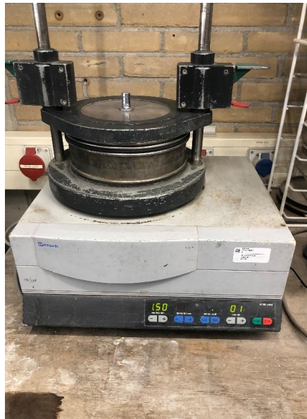
Image 1: disk mill to mill samples into powder. Image 2: Sieve shaker for homogeneity.
