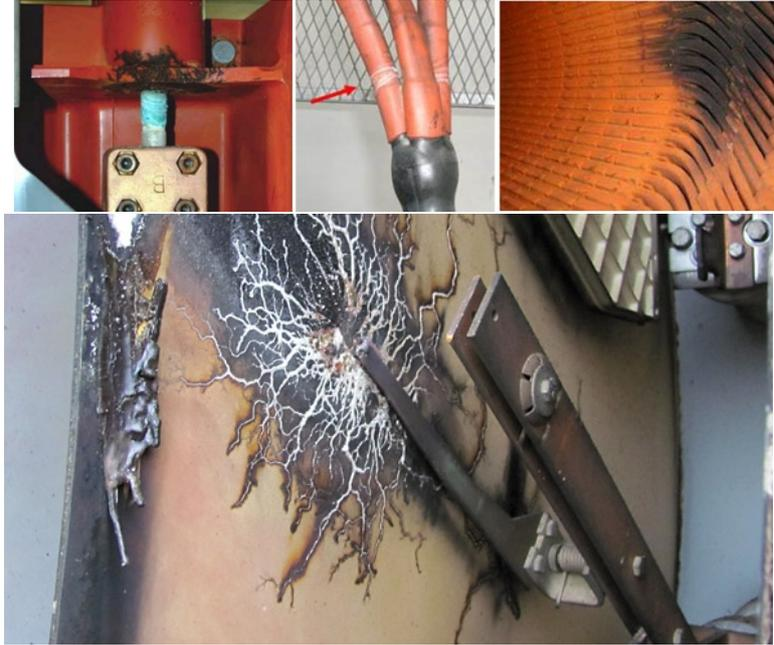
Figure 1.2: Deteriorating/Failing HV assets due to prolonged PD activity
