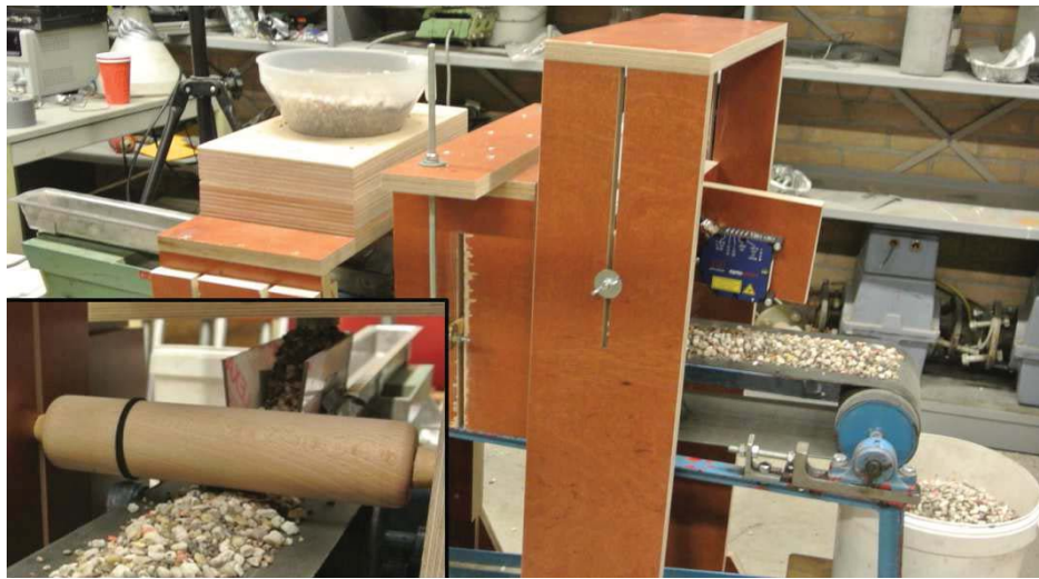
Figure 2. Conveyor setup for testing the gravel batches.
