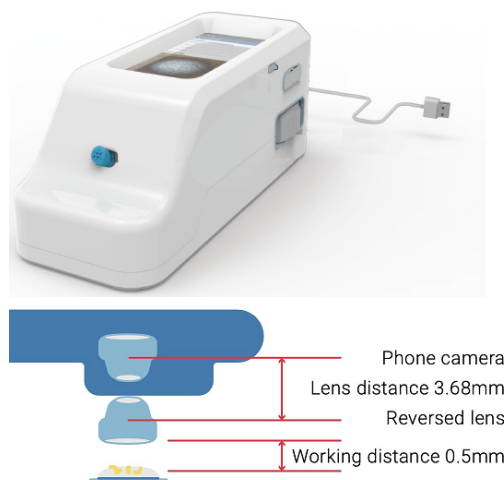
Fig. 4. Schistoscope SP (up) with working principle of sensor and lens combination (down)
