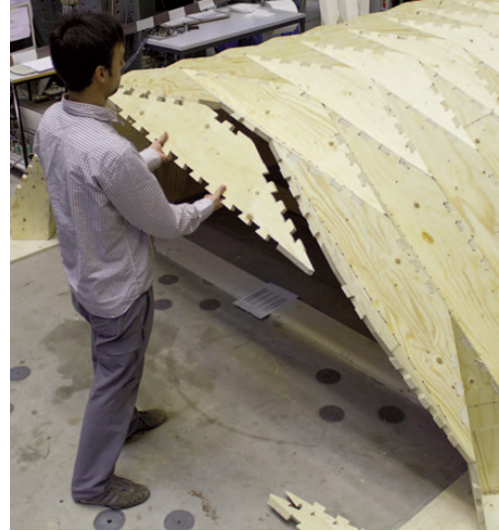
Figure 86: A dovetail joint to geometrically interlock structural wooden components (Robeller & Weinand, 2015)
