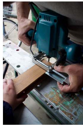
Figure 203: Milling the slots into the wooden insert (own work, 2025)
