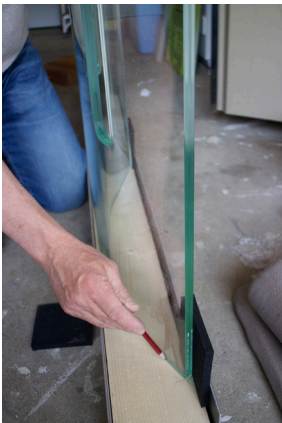
Figure 201: Marking the outlines of modules 1 and 2 on the lower spruce wooden board (own work, 2025)
