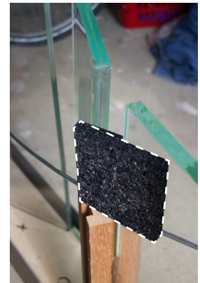
Figure 209: Rubber insert placed in the slot for clamping (own work, 2025)
