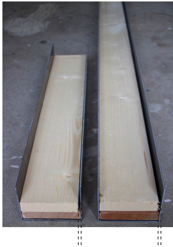
Figure 200: Spruce board cut to size, leaving space for a wedge (own work, 2025)
