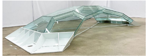
Figure 33: Modular glass bridge prototype (Lu et al., 2022).
