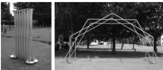
Figure 23: Scissor mechanism for a deployable structure (Brancart et al., 2017)
