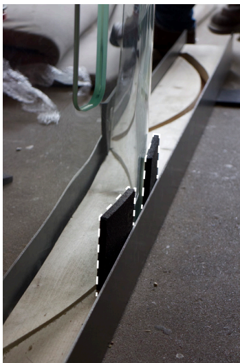
Figure 206: Clamping rubbers positioned between the glass and the steel U-profile (own work, 2025)
