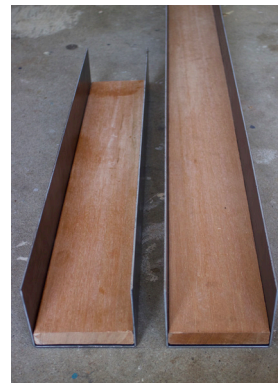
Figure 199: Hardwood clamped into the upper and lower U-profiles (own work, 2025).
