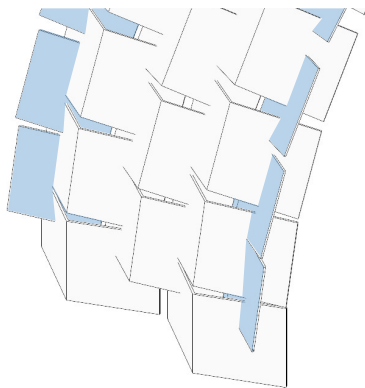
Figure 109: Side panels that have to be removed to extend the structure in the x-direction (own work, 2025)
