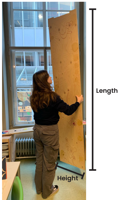
Figure 128: A long module with a limited height, to find a compromise between adaptability and manual assembly (own work, 2025)
