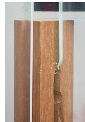
Figure 216: Small local failure in the hardwood slot around 8 kN (own work, 2025)
