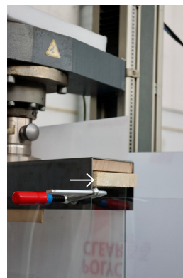
Figure 215: Spruce wood started moving around 8 kN (own work, 2025)
