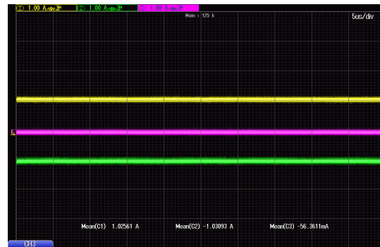
(b) Battery discharging 1.0 A into an electronic load via two converters
