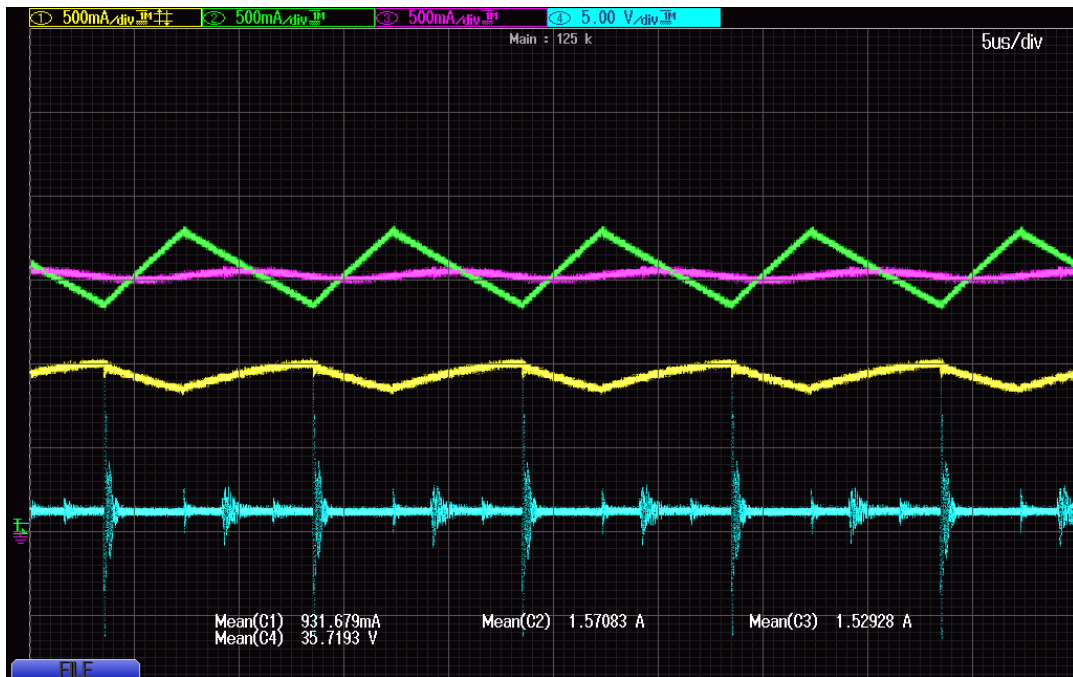
Figure A.6: DC Inductor current, battery voltage
