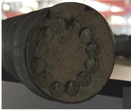
2 Figure 5. Detail of prestressing strands: sketch and photograph. Conversion: 1 mm = 0.04 in.
