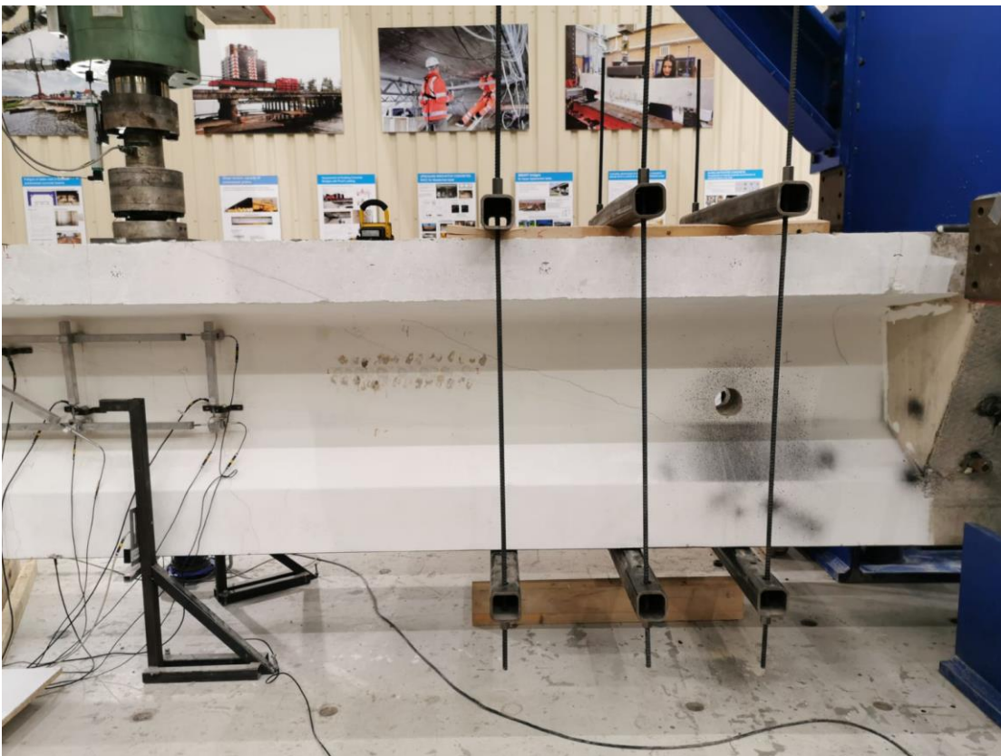
4 Figure 8. External transverse prestressing applied to avoid possible failure on the unwanted
