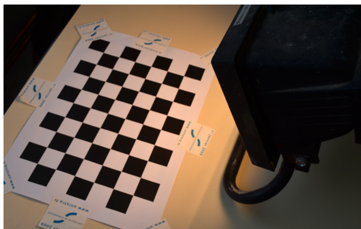
FIGURE 6.7: Set-up for obtaining thermal calibration images
