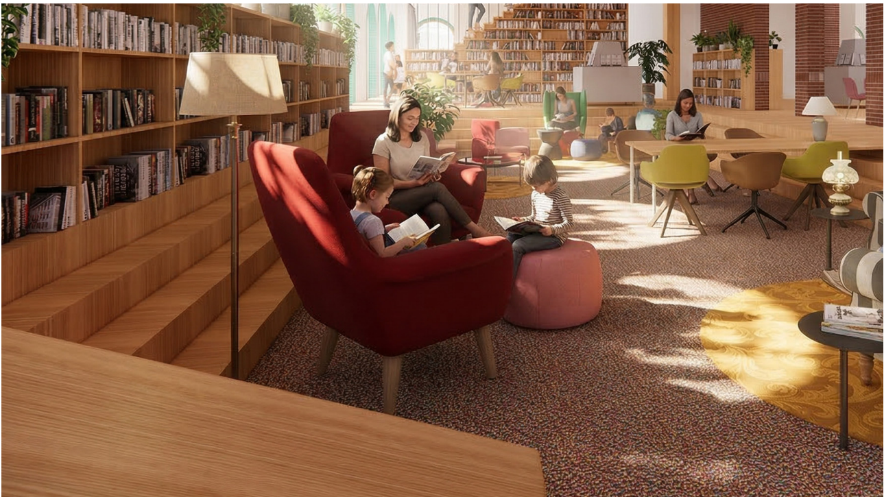
Figure 2.11: Lowered seating area (library) with wheelchair ramp and bookcases doubling as railing
