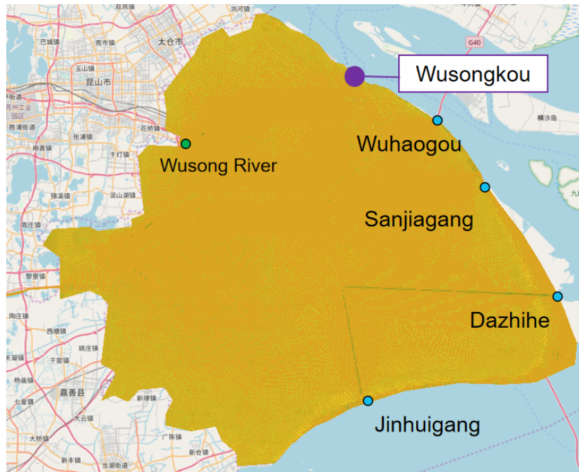
Fig. 3.13.: Overview of the computational grid in overland simulation. Blue points are the location of the sluices. The green point is the boundary point of Wusong River in the model
