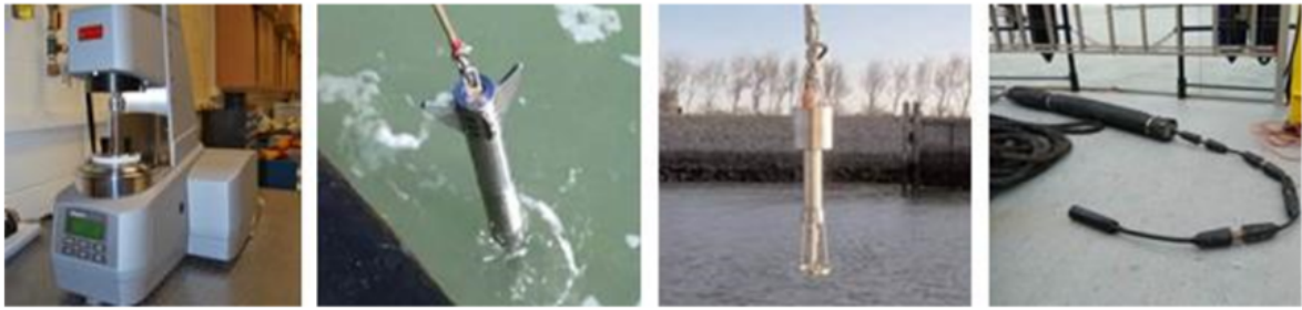
Figure 1.1: Examples of rheology-based methods. From left to right: lab rheometer, free falling cone (Graviprobe), tuning fork (Rheotune), towing object (Rheocable), (Kiricheck et al., 2018)
