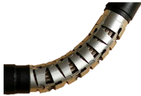
Figure 4: An up close view of the bending section of the cable ring grasper. [7].
