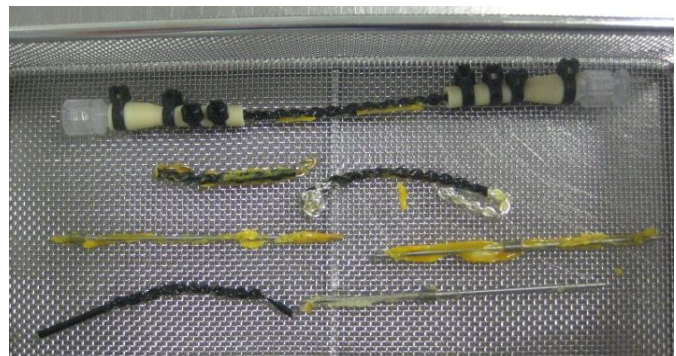
Figure 19: All the soiled test fixtures in a holding basket before being put through the washer disinfector.
