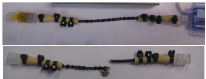
Figure 21: Images of the seal testing fixture before and after five autoclave cycles.
