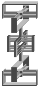
Figure 3.11: Flexural joints for the design of constraining legs for compliant parallel kinematic machines. Reproduced from [86].
