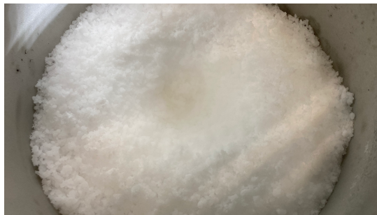
Figure 6.8: Crater in icy particles where the crater depth is shallow enough for the crater to be valid (drop #67).
