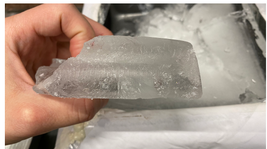
Figure 6.4: Cross-sectional view of shattered ice formed in metal container (drop #57).
