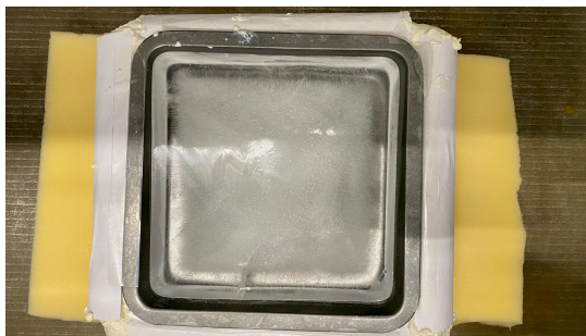
Figure 3.7: Square container, with insulating foam. Here pictured on top of the dampening foam.
