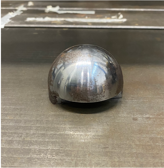
Figure 3.2: Spherical tip, 545.5 g of mass. Top outer diameter of 60 mm and tip radius of 30 mm. Tip identifier #6.
