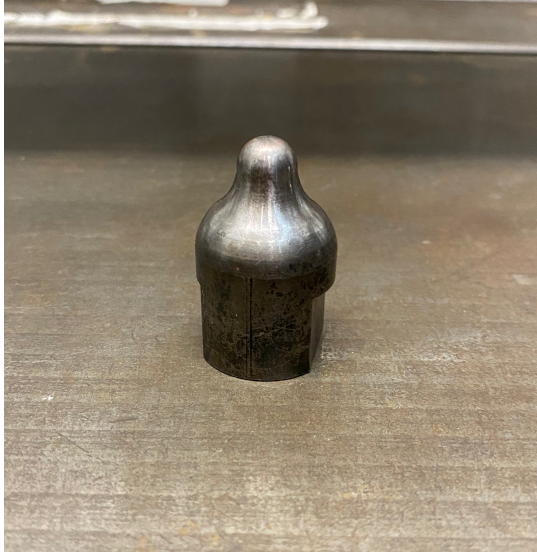
Figure 5.1: Bell-shaped tip, 86.5 g of mass. Top outer diameter of 25 mm and tip radius of 5 mm. Tip identifier #11.
