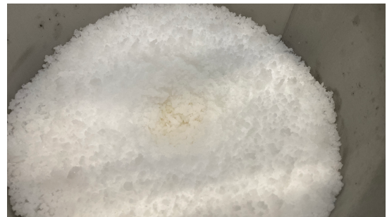
Figure 6.9: Crater in icy particles where the crater depth is too deep, making the crater invalid (drop #70).
