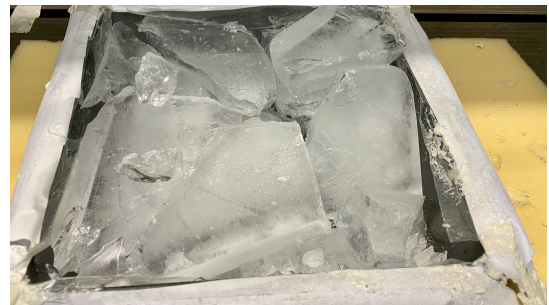
Figure 6.2: Shattered ice for the experiment performed with dampening foam, obtained for 51.6 J impact energy (drop #59).
