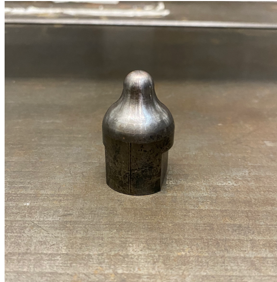
Figure 3.3: Bell-shaped tip, 86.5 g of mass. Top outer diameter of 25 mm and tip radius of 5 mm. Tip identifier #11.
