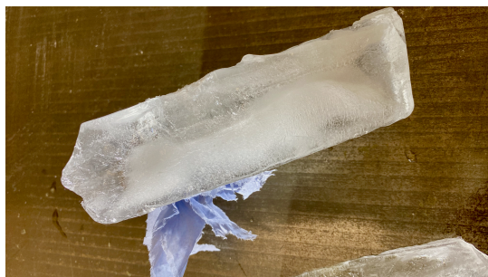
Figure 6.3: Cross-sectional view of shattered ice formed in plastic container (drop #45).
