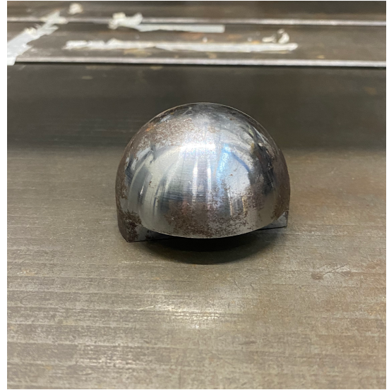
Figure 5.2: Spherical tip, 545.5 g of mass. Top outer diameter of 60 mm and tip radius of 30 mm. Tip identifier #6.
