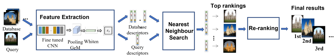
Figure 1.4: The pipeline of our image search engine. There are three main steps: feature extraction, NN search and re-ranking.
