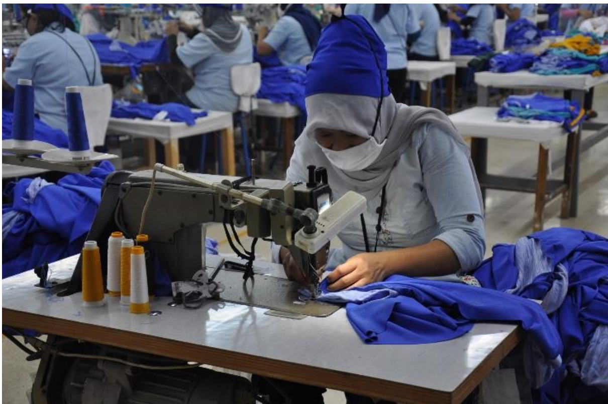
fig App.D.8 | sewing operator with an extra LED-lamp shining onto her hands (own image)
