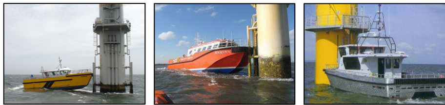
Figure 1.7 Ship-based access to offshore wind turbines Ships used: a) WindCat b) Aryan c) Valhalla
