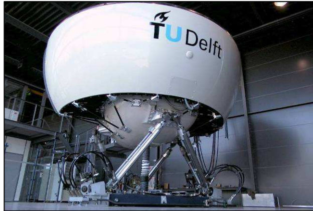
Figure 2.9 A flight simulator supported by a Stewart platform
