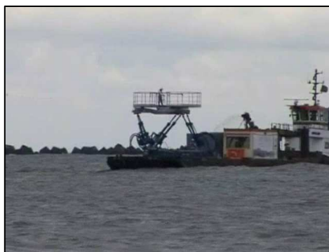
Figure 7.16 First motion compensation test
