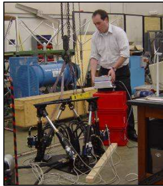
Figure 3.14 Testing of the control software by manipulating the Octans and visually checking the MMS motions
