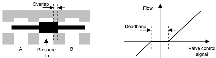
Figure 7.11 Characteristics of a valve with an overlap spool
