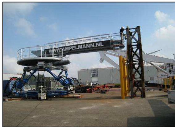
Figure 7.17 Operation simulation with full scale dummy boat landing
