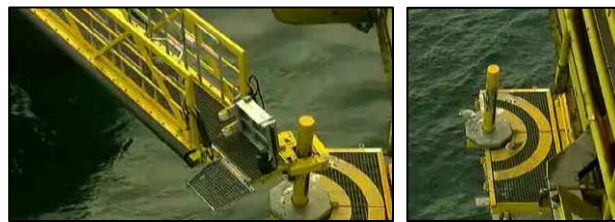
Figure 2.4 a) OAS connected to landing platform b) OAS landing platform
