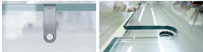
Figure E.8: Cutouts in laminated glass [86]
