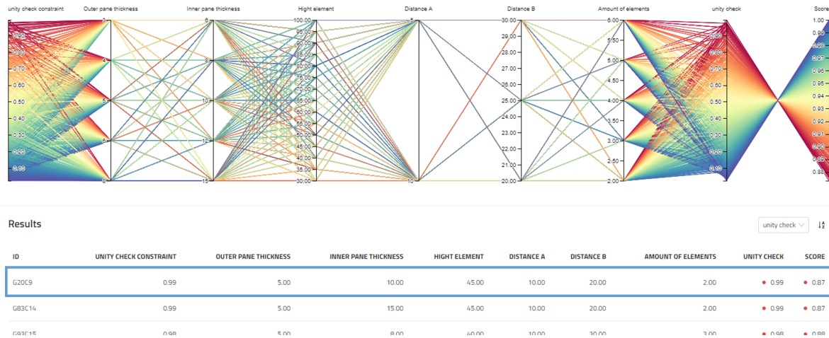
Figure D.25: Autostudy results for the dimensioning of detail D. Parameters from left to right: Unity check constraint; Outer pane thickness; Inner pane thickness; Height element; Distance A; Distance B; Amount of elements; Unity check; Score.
