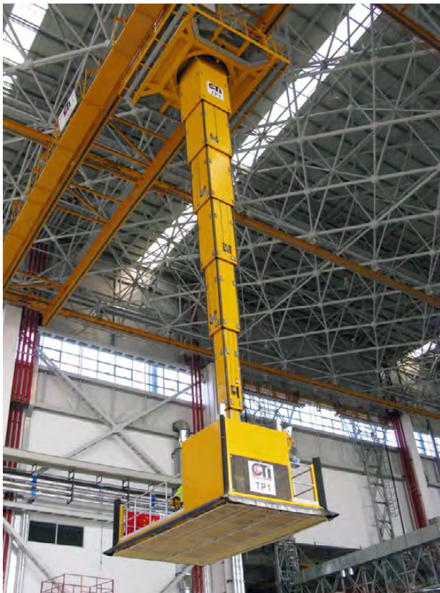
Teleplatforms in use in a hangar in South Korea for maintenance of Airbus A380 (CTI Systems, n.d.)
