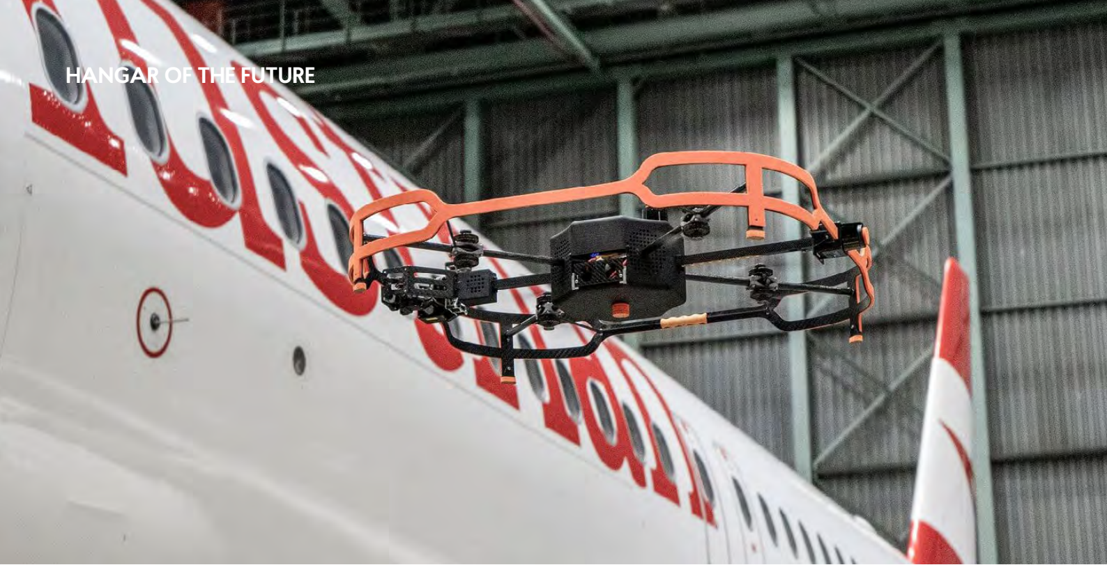
Austrian Airlines testing drone inspection (Aamir, 2019)
