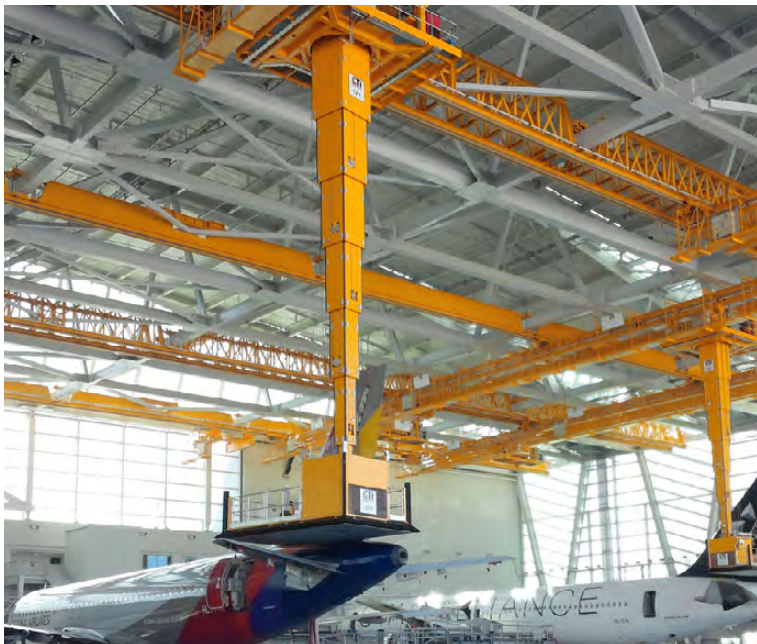
Teleplatforms in use in a hangar in South Korea for maintenance of Airbus A380 (CTI Systems, n.d.)
