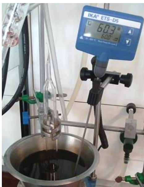
Figure 6.1. A typical setup for free radical polymerization with flame sealed polymerization tube.
