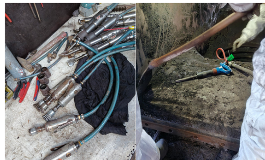
Fig. 15: Mechanical tools used in the mechanical removing task. (Top-left) Small handheld mechanical chisels that vibrate. (Bottom-left) Handheld Mechanical sanding tool that rotates. (Right) Big handheld mechanical chisel.
