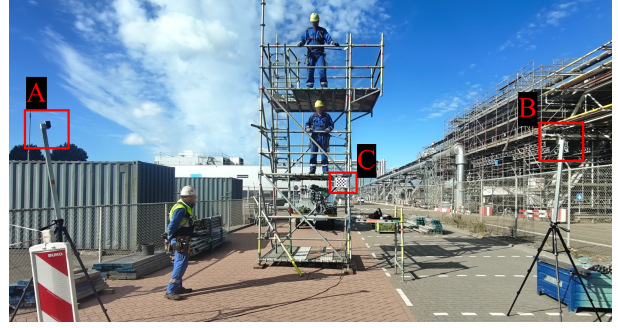
Fig. 4: Experimental Setup for the POT, using a two-story scaffold setup. (A) and (B) iPhone cameras, (C) Rastergrid used for the calibration of the cameras.
