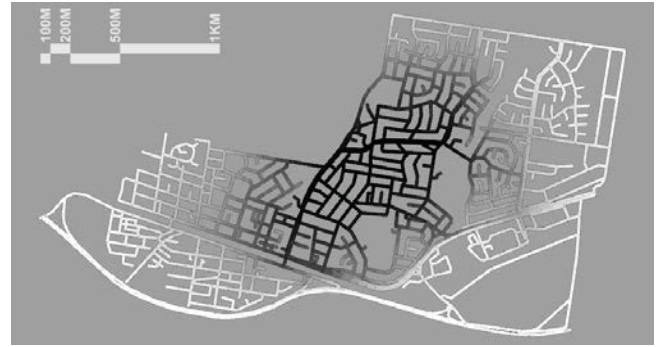
Figure 12. Eigenvector Centrality index of the Closeness matrix, when distances above “25 minutes cycling” are considered ‘far’
