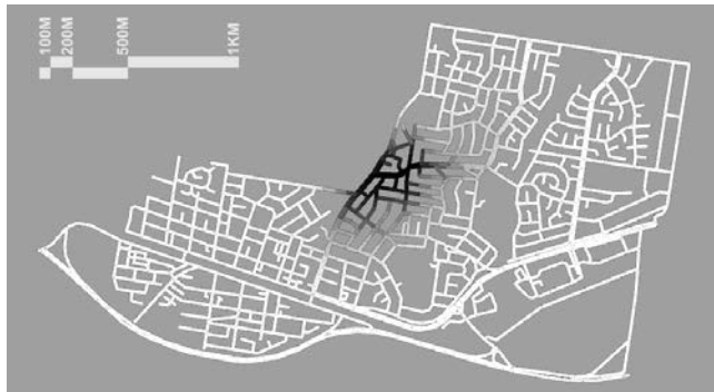
Figure 10. Eigenvector Centrality index of the Closeness matrix, when distances above “10 minutes cycling” are considered ‘far’
