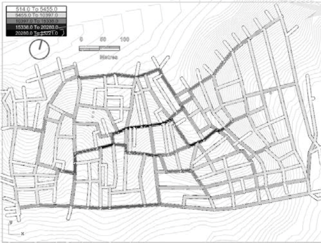
Figure 4. Easiest Paths Betweenness Centrality, \tau = 15' , Directed Graph, Search Radius is 10 Minutes Walking
